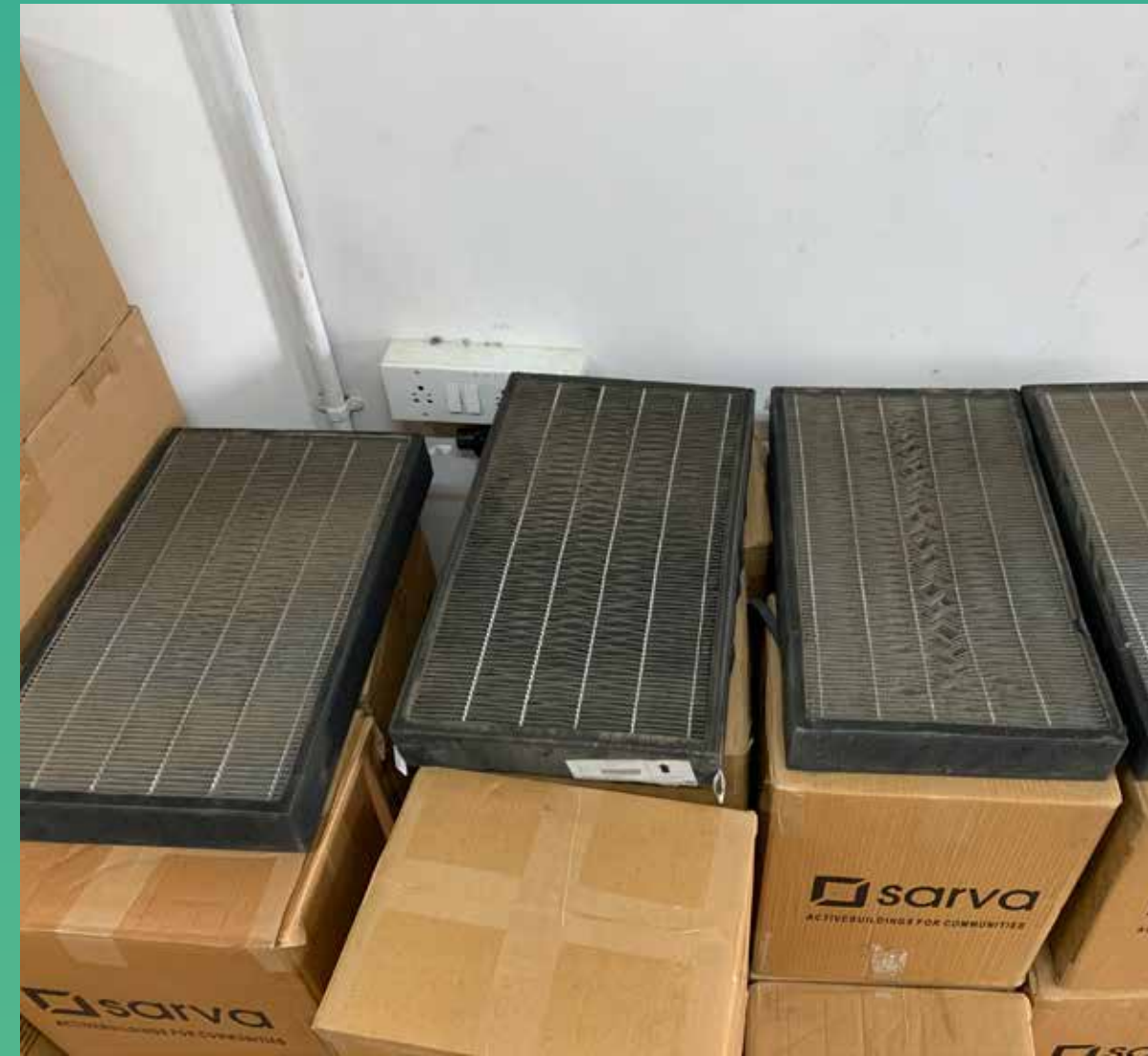
Rapidly Deteriorated Filters
